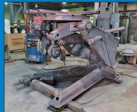
9,000 Lb. P&H Model WP-6 Motorized Tilting & Rotating Welding Positioner
