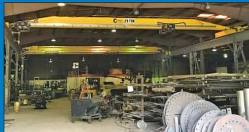
20 Ton X 55' X 176' Free Standing Crane System w/20 Ton and 15 Ton Bridges
